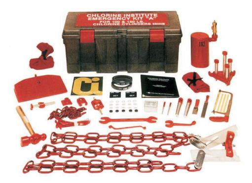
The Chlorine Institute Emergency Kit "A" is manufactured to the design specifications of the Chlorine Institute. The Emergency Kit "A" contains devices to stop leaks at the valve, fusible plug, and in the side walls of chlorine 100 & 150 lb. cylinders which conform to specification DOT 3A480. Two instruction booklets explaining the application of each device are included.
