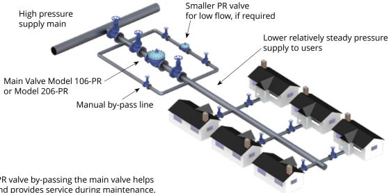
Note: The smaller PR valve by-passing the main valve helps control low flows and provides service during maintenance. It should be set 3-5 psi / 0.2-0.35 bar higher than the larger valve setting.
